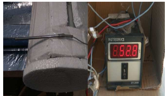
FIG. 3. PENCIL TYPE THERMOCOUPLE AND TEMP. INDICATOR
