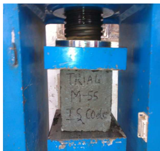
Fig No.1: Testing of cubes
