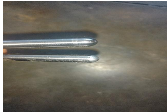
Figure 3. 8 mm & 12 mm H.S.S tool
