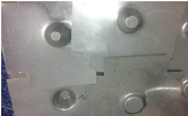
Figure. 5 Sheets having fracture at certain wall angle in SPIF process
