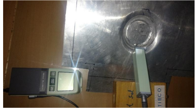
Figure 6 Surface measurement through Mitutoya surf-test SJ-201P
