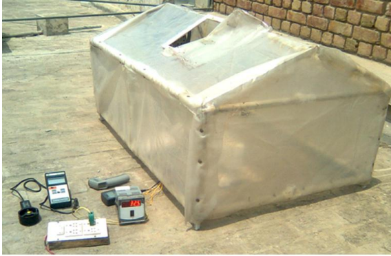
Fig. 3 Photographic view of orangery drying under natural convection
