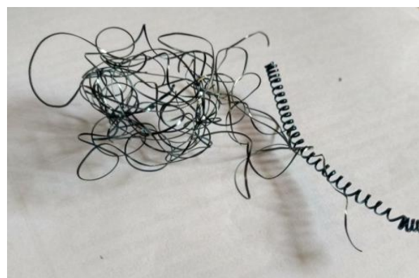
Fig. 8: Actual Chips Formed in Dry Machining
