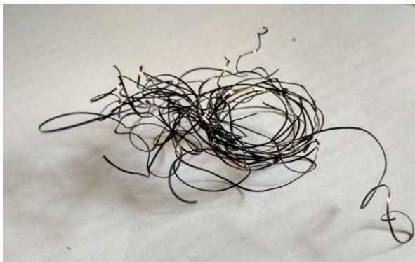
Fig. 10: Actual Chips Formed in MQL Machining
